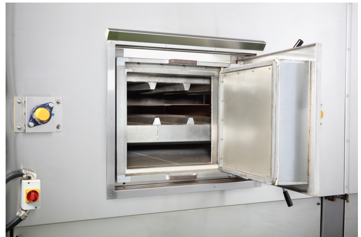
Hinged access door showing top and bottom impingement nozzles
